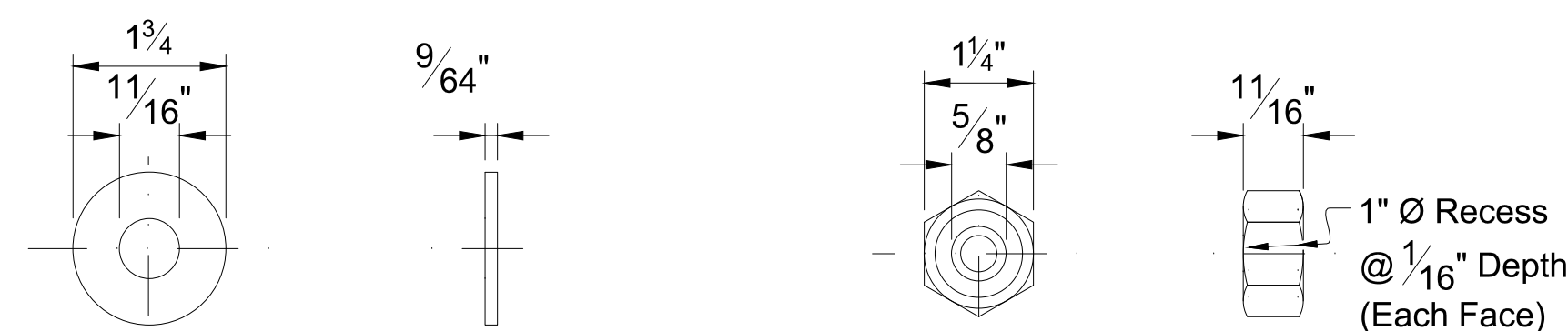
ELEVATION PROFILE ELEVATION PROFILE WASHER HEX-NUT
